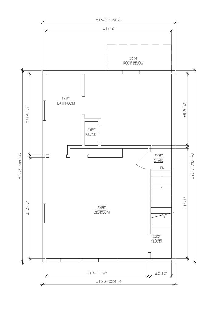
$\frac{2ND FLOOR PLAN (EXISTING)}{SCALE: 1/4" = 1'-0"}$
