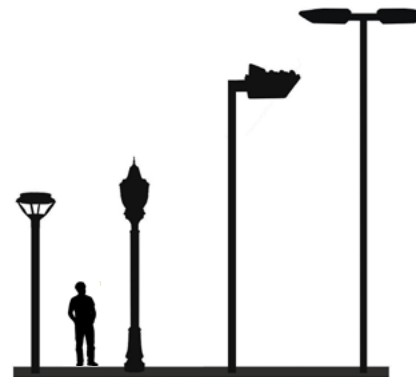
Lighting pole styles and height
