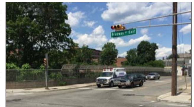
Intersection of Freeway Drive East and South Day Street (No ADA ramps on north side of intersection)
